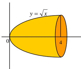
$$\begin{aligned} V &= \pi \int_0^4 (\sqrt{x})^2 \cdot dx = \pi \int_0^4 x \cdot dx = \pi \cdot \left[ \frac{x^2}{2} \right]_0^4 = \\ &= \pi \cdot \left( \frac{4^2}{2} - 0 \right) = 8\pi \text{ u.v.} \end{aligned}$$
