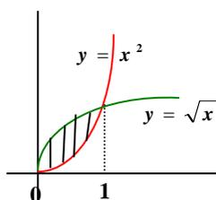
$$\left. \begin{array}{l} y = x^2 \\ y^2 = x \end{array} \right\} \Rightarrow (x^2)^2 = x \Rightarrow x^4 - x = 0 \Rightarrow x(x^3 - 1) = 0 \Rightarrow \begin{cases} x = 0 \\ x = 1 \end{cases}$$
