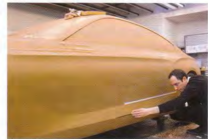
Clay model of a new car design
